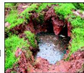
Figure 4. This photograph shows a concrete septic tank lid that has collapsed under a truck's weight. Repair costs were more than $1,000.
